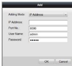
Figure 5-8 Adding by IP Address
